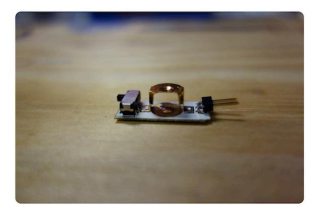
Turn on the switch by flipping the lever up, and measure the voltage across the 2-pin header, the reading should be around 3.1V.
