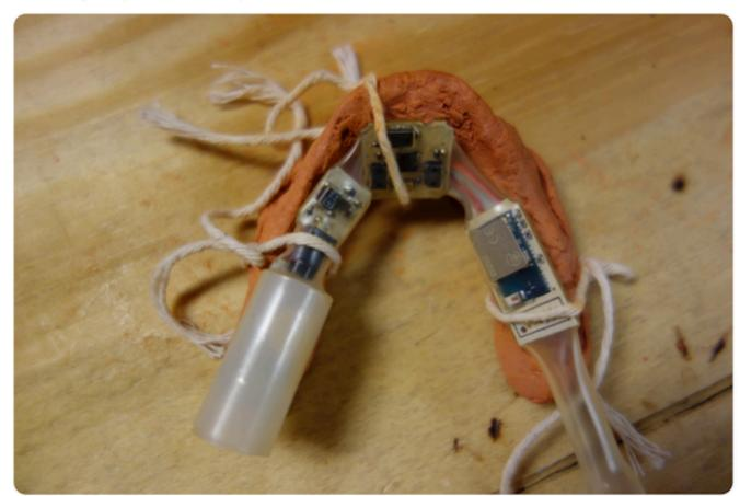
Heat everything up with a heatgun until full shrinkage. While the end of the heatshrink tubing is heated (feels rubbery) and open on the microcontroller side, clamp it shut with tweezers to seal it. Inspect the seal and cut off excess heatshrink.
