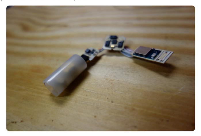
Carefully slide the Sensor Ribbon with battery cover tube into the heatshrink tubing.
